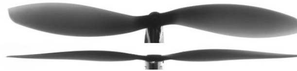
Figure 1: APC Slow Flyer 10x4.7 rotor (top and side view)
