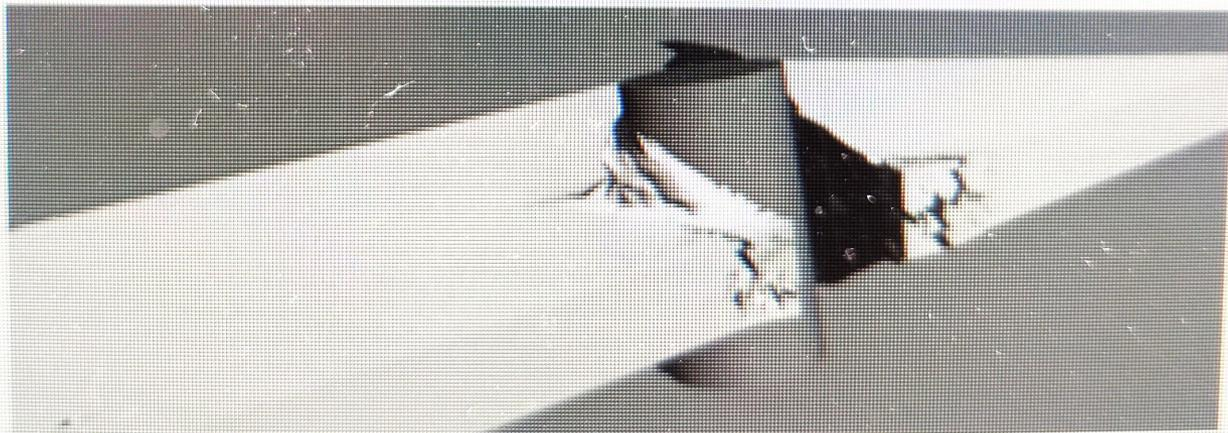
Fig. 5. Pattern of ice floe destruction during collision with offshore structure.
